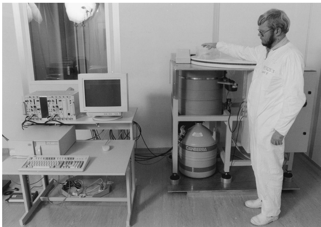
Fig. 3. High-resolution \gamma -spectrometer for screening swipe samples.
