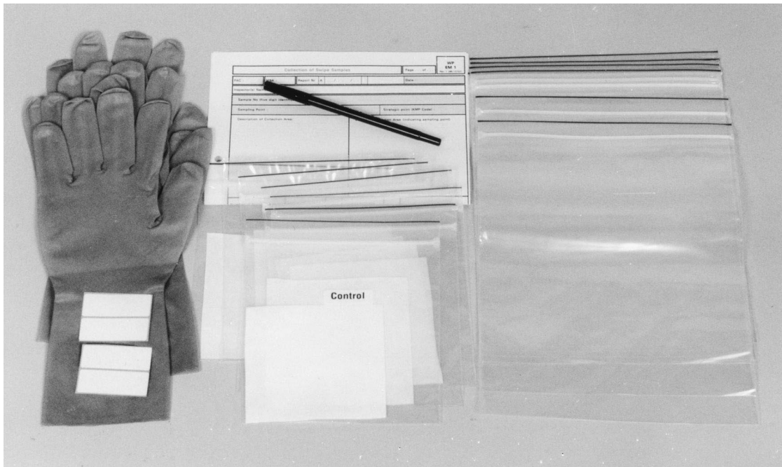
Fig. 1. IAEA cotton swipe sampling kit.
